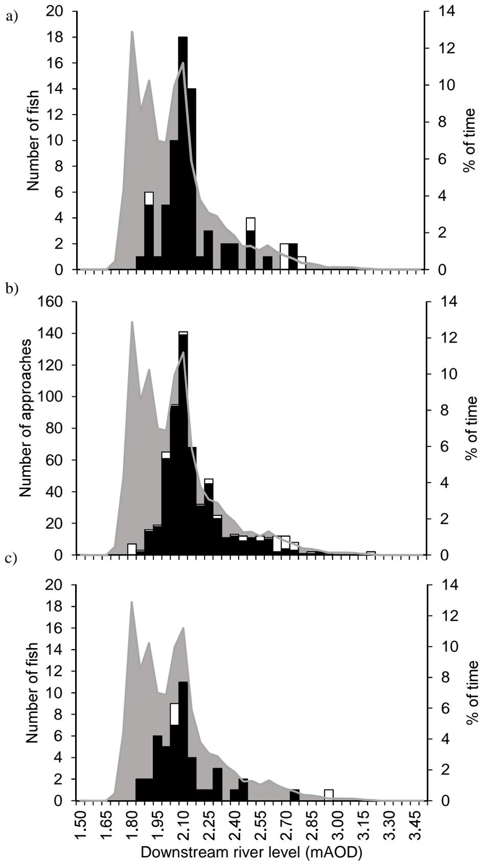
Figure 4: Relationship between downstream river level (mAOD) and first AST/FPS approach (a), subsequent non-passage AST/FPS approaches (b) and FPS passage (c) during periods when the hydropower is on (black) and off (white).
