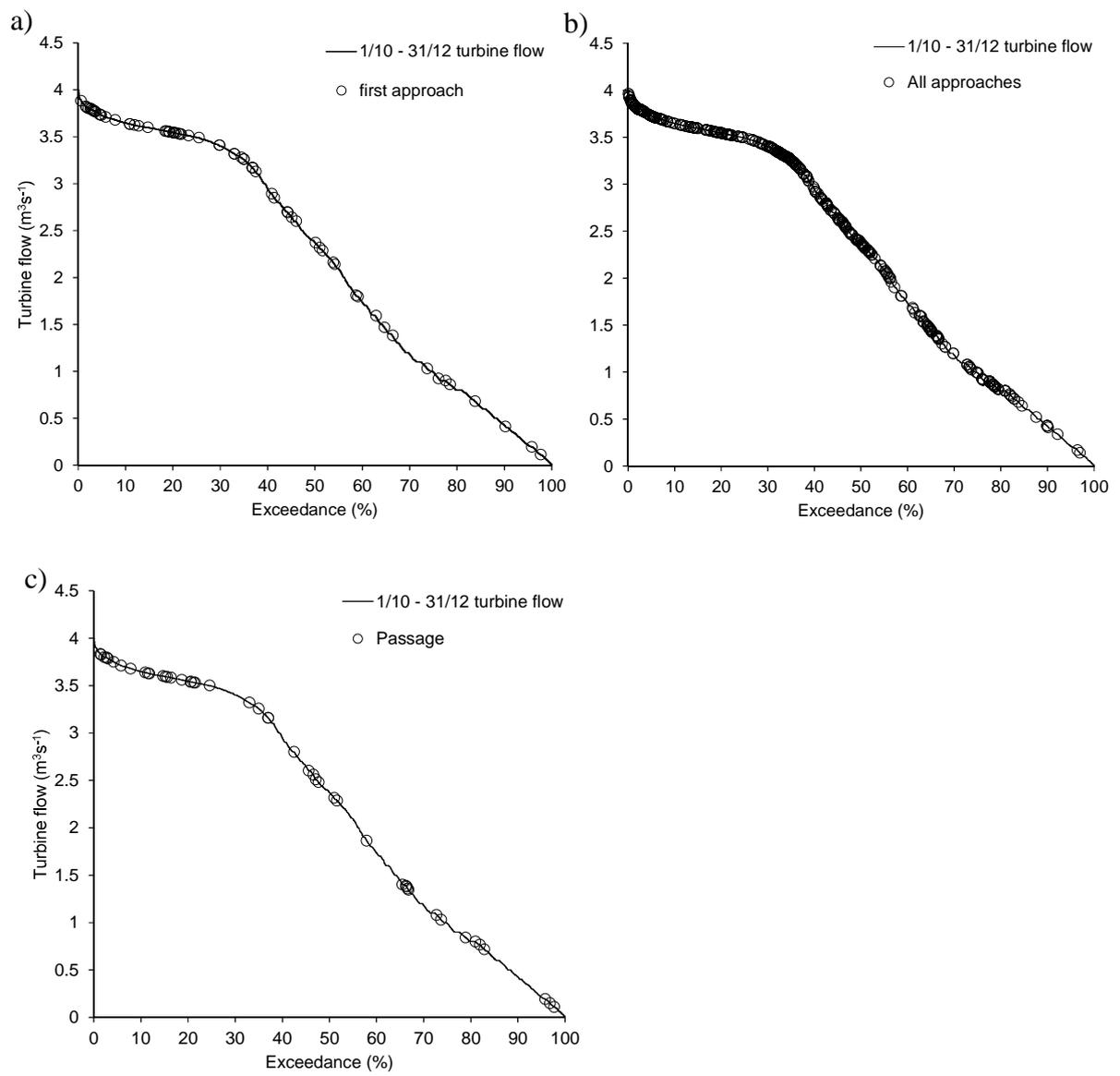
Figure 5: First AST/FPS approaches (a), subsequent non-passage AST/FPS approaches (b) and FPS passages (c) in relation to AST flow exceedance curves during operation (i.e. turbine flow = 0, not plotted).
