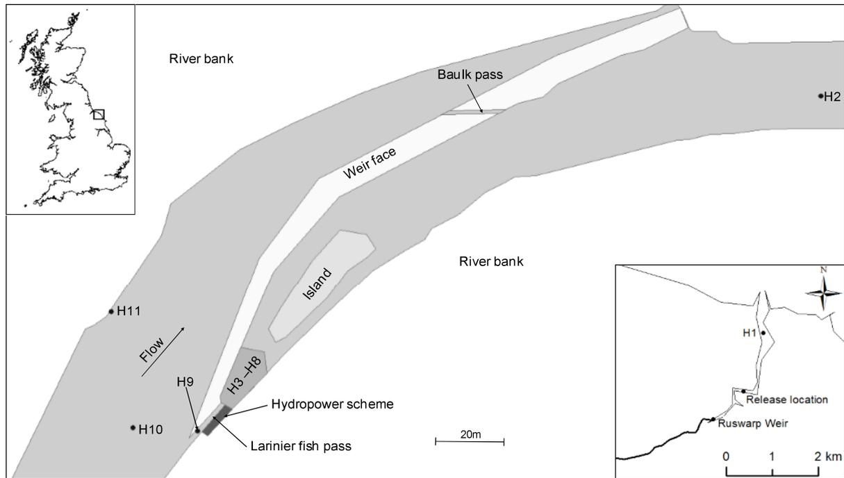
Figure 1: A map of Ruswarp Weir on the Yorkshire Esk, England, including the location of fish passes, hydropower scheme and monitoring equipment (hydrophones H1-H11).
